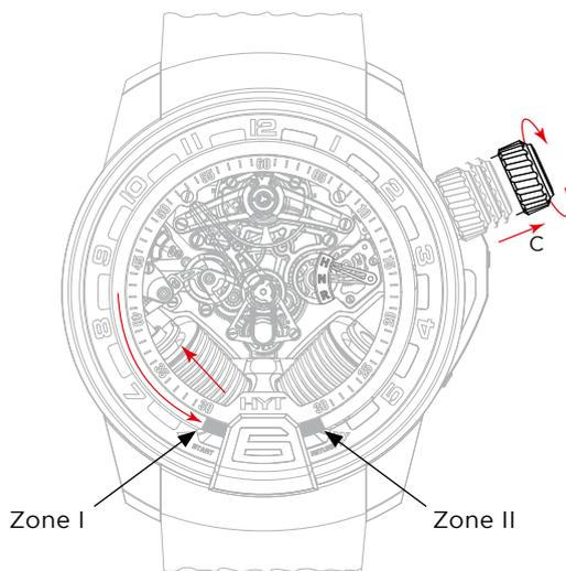
**Important :** If you plan to not wear the watch for a while, the coloured liquid has to be stored in its own reservoir (on the left bellows<sup>2</sup>).
