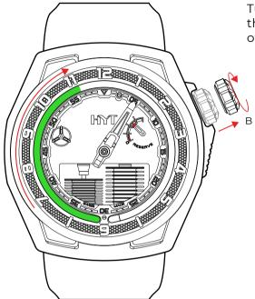
Turning the crown once is the equivalent of a change of around 15 minutes.
