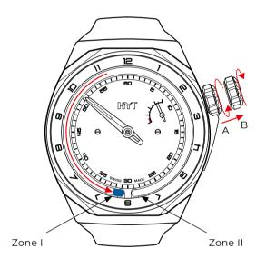
Important: if you do not intend to wear the watch for some time, the coloured liquid must be kept in its own Below (left piston).
