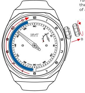
Turning the crown once is the equivalent of a change of around 15 minutes.
